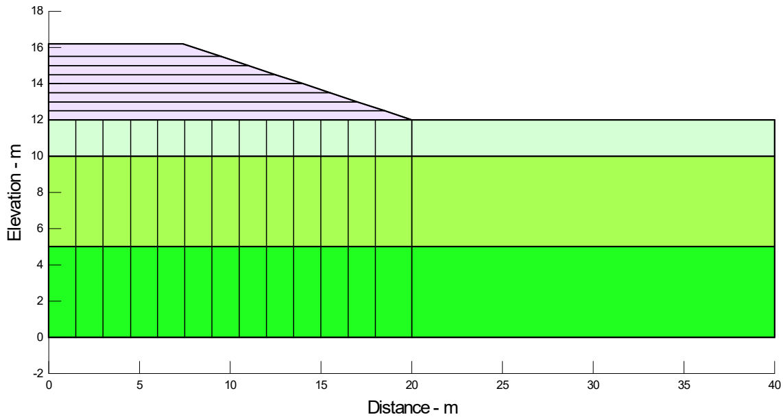
Figure 2. Position of the vertical drains and layers used for sequential fill placement.
