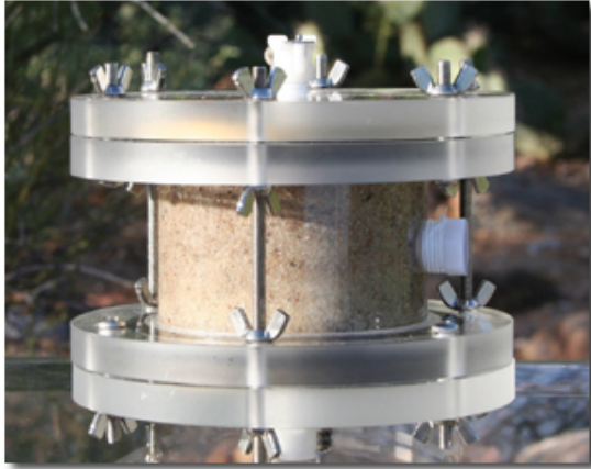
Figure 1. Tempe cell by Soil Measurement Systems ( http://www.soilmeasurement.com/tempe.html ).
