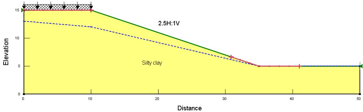
Figure 1. The geometry of the cut slope.
