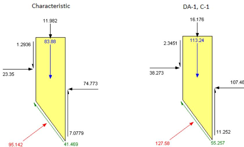
Figure 7. Slice weights and surcharge loads of Slice 3.
