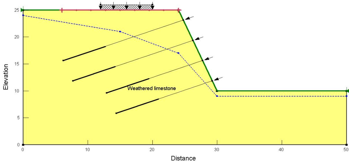
Figure 2. Geometry of the limestone slope.
