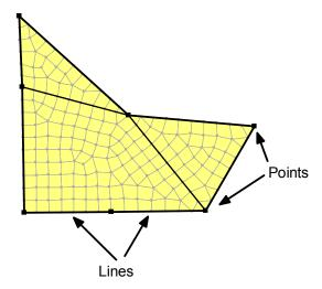
Figure 3-5 Illustration of a region's lines and points
