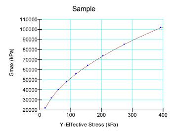
Figure 4-7 A typical G<sub>max</sub> function for cohesive soil
