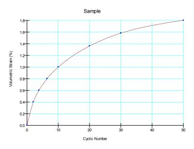
Figure 4-23 Volumetric strain versus shear cycles
