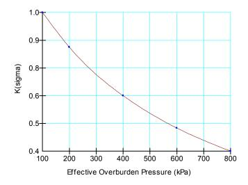
Figure 4-16 A typical K<sub>s</sub> correction function
