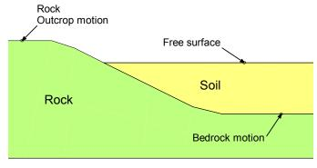
Figure 5-4 Definition of motion types
