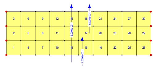
Figure 2-16 Horizontal flow through three element section
