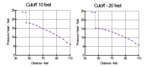
Figure 2-7 Uplift pressure distributions along base of structure
