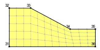
Figure 3-20 Rectangular grid of quad elements
