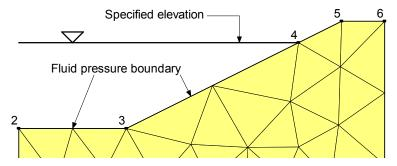
Figure 5-11 Illustration of fluid pressure boundary
