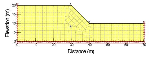
Figure 5-9 Illustration of fixed boundary conditions
