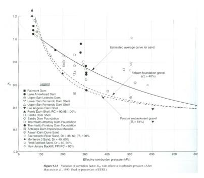
Figure 4-17 Overburden correction factor K<sub>s</sub>
