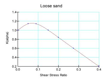
Figure 4-19 Shear stress correction function
