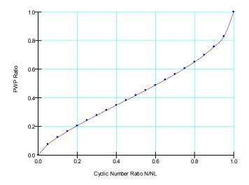
Figure 4-13 Cyclic number ratio N/N<sub>L</sub> versus pore pressure ratio r<sub>u</sub>
