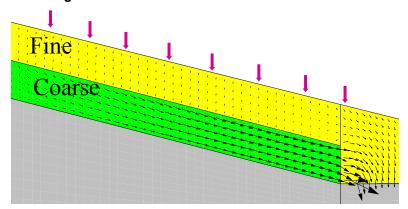
Figure 2-12 Flow diversion under high infiltration
