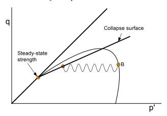
Figure 1-6 Cyclic stress path from B to the collapse surface
