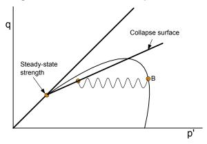
Figure 4-27 Stress path onto the collapse surface during cyclic loading
