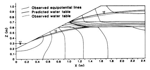
Figure 2-1 Rulon's laboratory scaled model results
