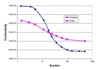
Figure 2-10 Hydraulic conductivity functions
