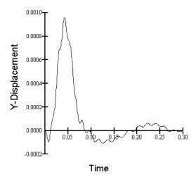
Figure 5-15 Displacement from a velocity time history record
