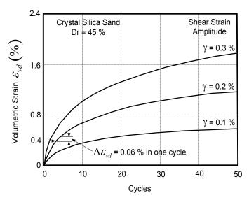
Figure 4-22 Volumetric strain curves for constant cyclic shear strain amplitudes (after Martin et al., 1975)
