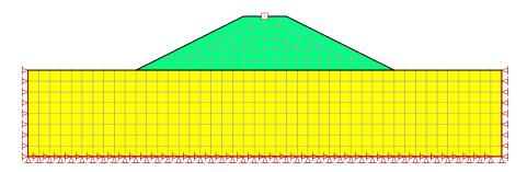
Figure 6-8 Illustration of displacement boundary conditions
