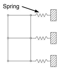
Figure 5-13 Spring boundary conditions
