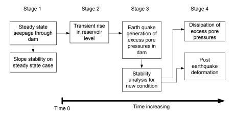
Figure 6-9 Example of staged work flow
