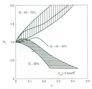
Figure 9.32 Variation of correction factor,  $K_{\alpha}$ , with initial shear/normal stress ratio. (After Seed and Harder, 1990. *H. Bolton Seed Memorial Symposium Proceedings*, Vol. 2, p. 364. Used by permission of BiTech Publishers, Ltd.)
