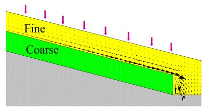
Figure 2-11 Flow diversion under low infiltration
