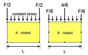
Figure 5-10 Stress equivalent nodal forces
