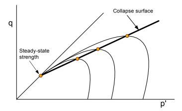
Figure 1-3 Collapse surface illustration
