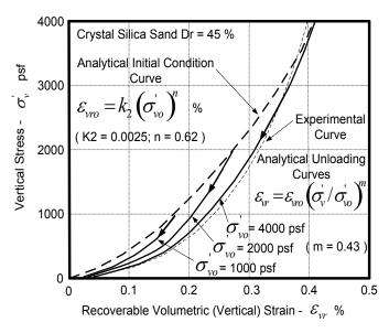
Figure 4-20 Recoverable strain unloading curves (after Martin et al., 1975)
