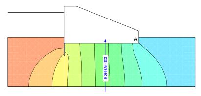
Figure 2-6 Seepage analysis with a cutoff
