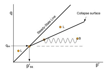
Figure 4-29 Liquefiable zones in q-p' space
