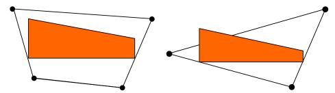
Figure 3-29 Primary field variable distribution in first-order elements
