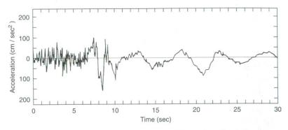
**Figure 9.45** Accelerogram from site near apartment building resting on liquefiable soil (shown in Figure 1.6) in 1964 Niigata earthquake. (After Aki, 1988.)
