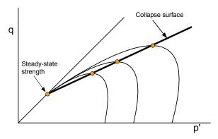
Figure 4-26 Definition of collapse surface
