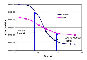
Figure 2-13 Conductivities under low and intense infiltration
