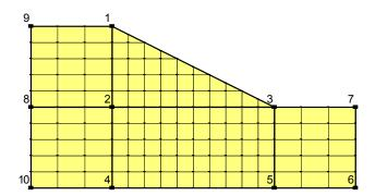
Figure 3-16 Structured mesh
