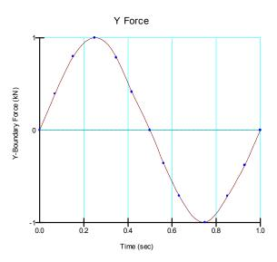
Figure 5-8 Example of a nodal force function
