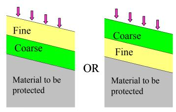
Figure 2-9 Two possible earth cover configurations
