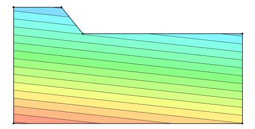
Figure 6-2 Spatial function assigned for initial pressures
