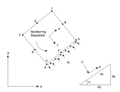
Figure 11-1 Normal and tangential pressure along an element edge
