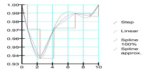
Figure 7-5 Comparison of all data point functions
