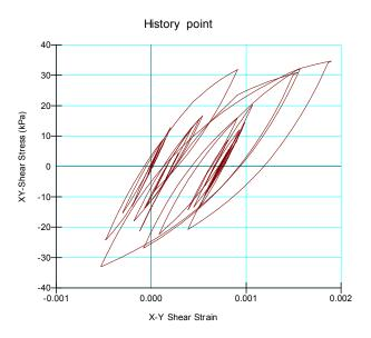
Figure 4-5 An illustrative QUAKE/W stress-strain curve
