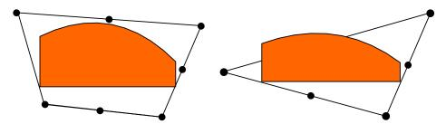
Figure 3-30 Primary field variable distribution in higher-order elements
