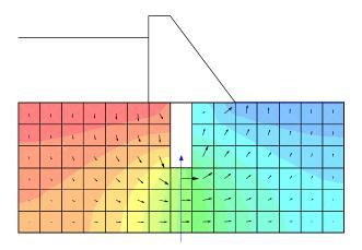
Figure 2-17 Simple flow beneath a cutoff
