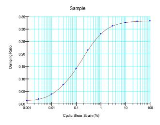
Figure 4-9 A damping ratio function
