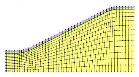
Figure 3-24 Mesh showing rounded surface slope breaks
