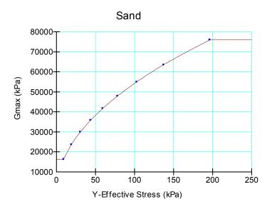
Figure 4-6 Typical G<sub>max</sub> function
