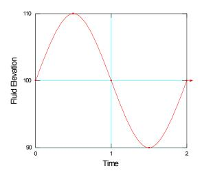
Figure 5-12 Fluid pressure boundary function
