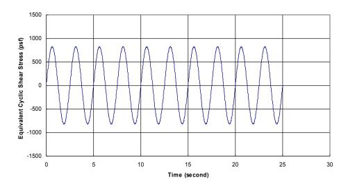
Figure 4-12 Equivalent cyclic shear stress
