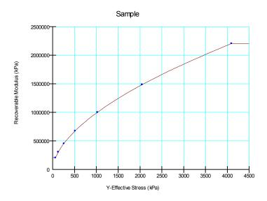
Figure 4-21 Recoverable modulus function
