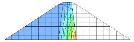
Figure 2-19 Head loss through dam core with downstream shell
