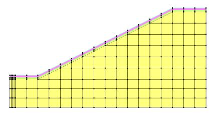
Figure 3-25 Mesh showing angular surface slope breaks
