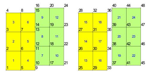
Figure 3-31 Disconnected elements - lack of compatibility
