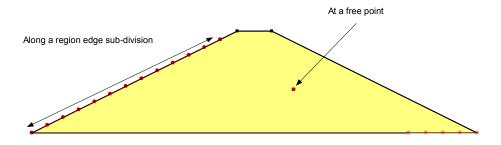
Figure 5-6 BC's attached to geometry
