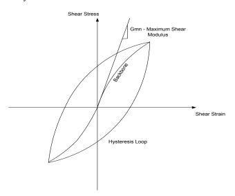
Figure 4-4 Hyperbolic backbone curve
