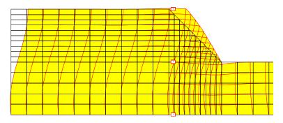
Figure 9-18 A deformed mesh at a 50x exaggeration
