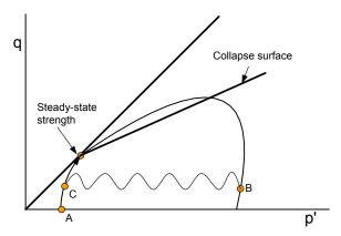
Figure 4-28 Stress path for dilative sands during cyclic loading
