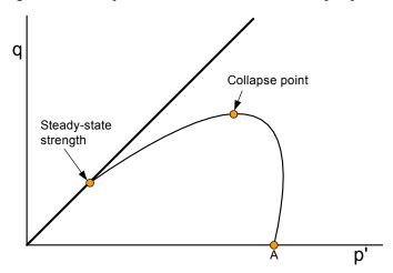
Figure 1-2 Effective stress path for loose sand under monotonic loading
