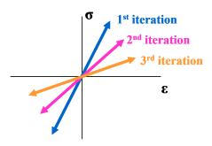
Figure 4-1 Change in G with each iteration through the earthquake
