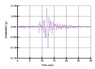
Figure 5-3 An earthquake record with a baseline correction
