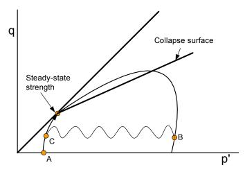
Figure 1-8 Stress path for cyclic loading with starting static stress state below steady-state strength
