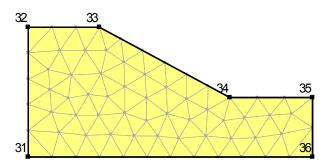
Figure 3-18 Unstructured triangular mesh
