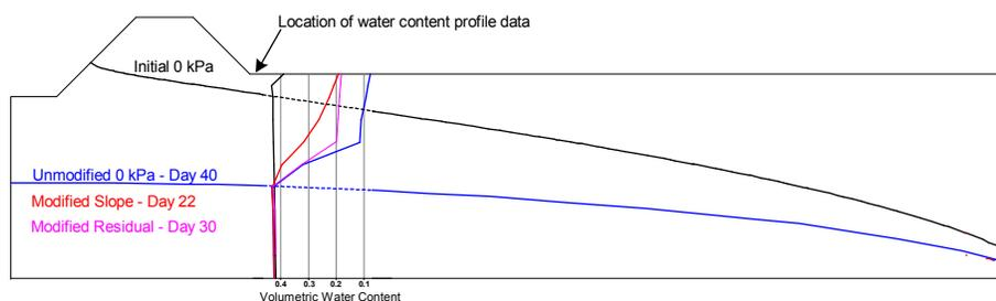
**Figure 2-25 Location of  $P=0$  kPa contours and water content profiles for the modified slope function (day 22), the modified residual (day 30) and the unmodified function (day 40)**
