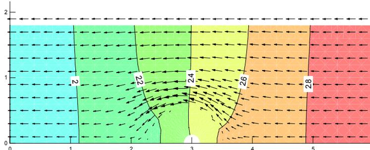
Figure 2-7 Seepage diversion around actively freezing soil region (Head contours from SEEP/W displayed)
