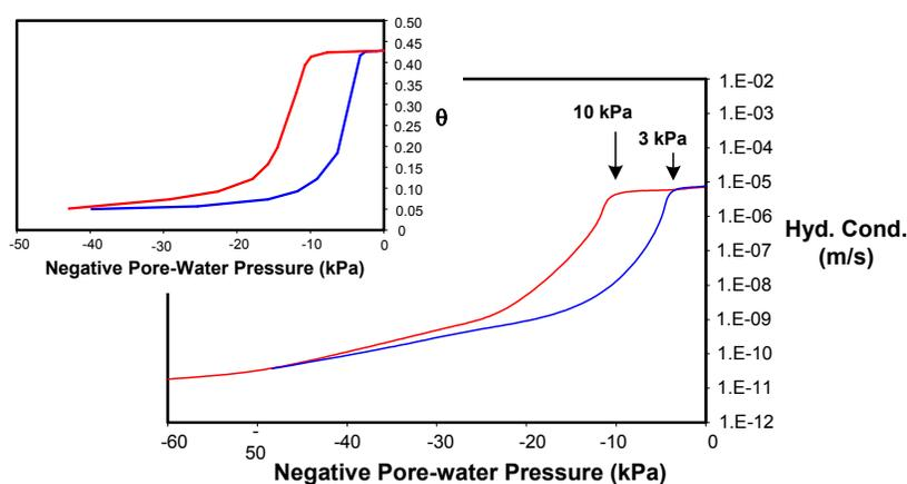
**Figure 2-12 Material property functions used in the AEV sensitivity analyses**
