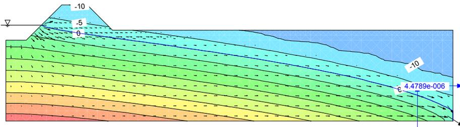
**Figure 2-20 Simulation #5 pressure head contours ( $K_{sat} = 7.5 \times 10^{-6}$  m/s)**
