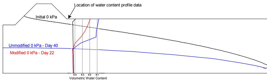
**Figure 2-23 Location of  $P=0$  kPa contour and water content profiles for the modified function (day 22) and unmodified function (day 40)**
