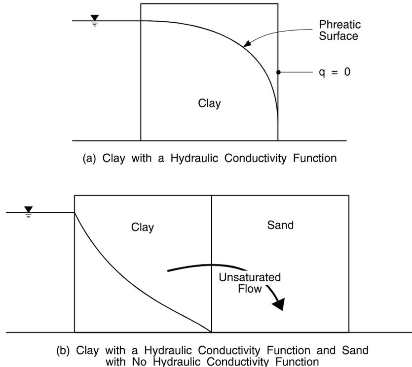
**Figure 2-5 Comparison of flow with and without a K function**
