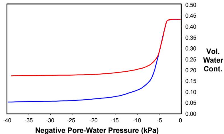
**Figure 2-24 Modified and unmodified residual water contents used in analyses**
