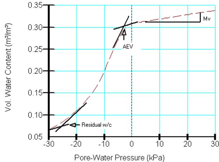
**Figure 2-1 Volumetric water content (storage) function**
