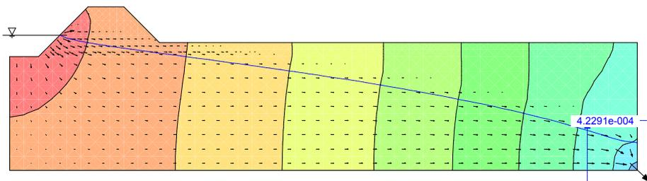
**Figure 2-16 Simulation #1 total head contours ( $K_{sat} 7.5 \times 10^{-4}$  m/s)**
