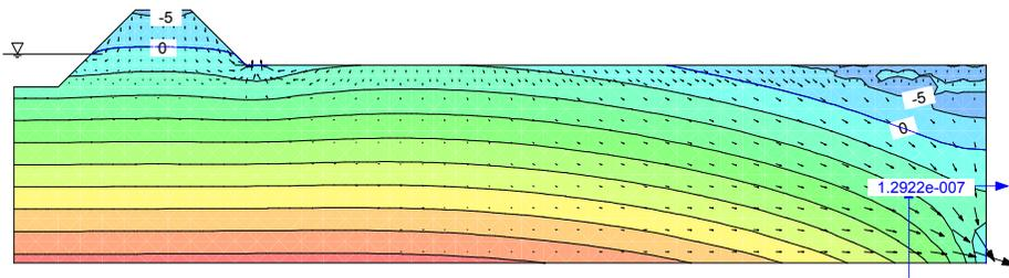
**Figure 2-21 Simulation #6 pressure head contours ( $K_{sat} = 7.5 \times 10^{-8}$  m/s)**
