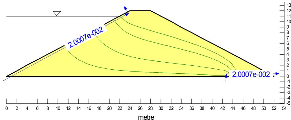
**Figure 7-13 Flux section used to check balance of inflow and outflow**
