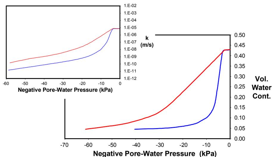
**Figure 2-22 Material property functions used in the sensitivity analyses for changes to the slope of the storage function**
