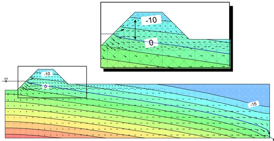
Figure 2-14 Pressure contours and flow vectors for a 10 kPa AEV material
