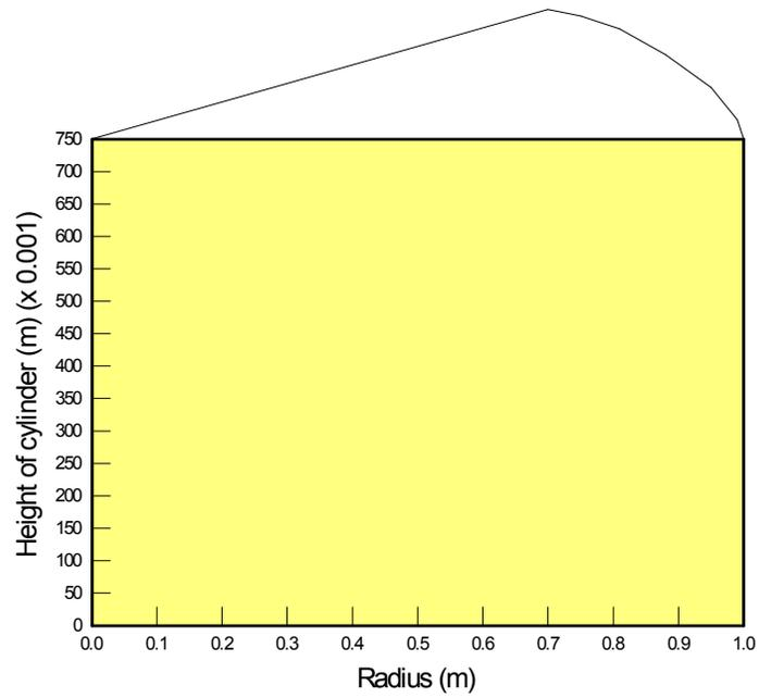
**Figure 4-3 Unit radian thickness in axisymmetric view**
