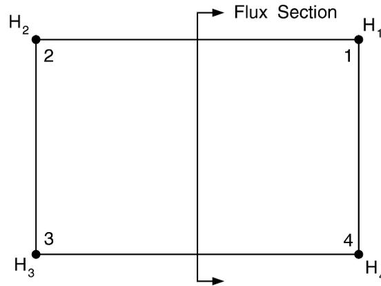
**Figure 7-12 Illustration of a flux section across a single element**
