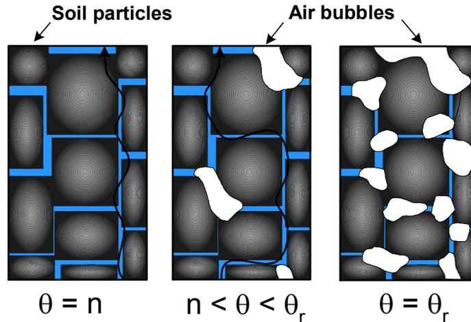
**Figure 2-4 Availability of water filled flow paths from saturation to residual**
