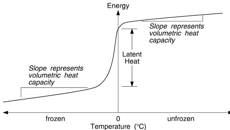
**Figure 2-10** An example of an energy storage function
