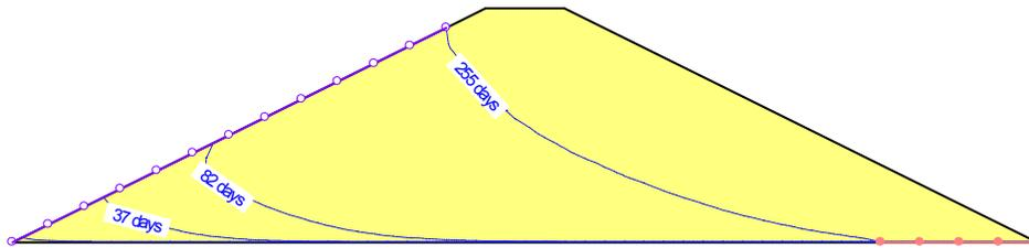
Figure 7-8 Water table (isolines) over time
