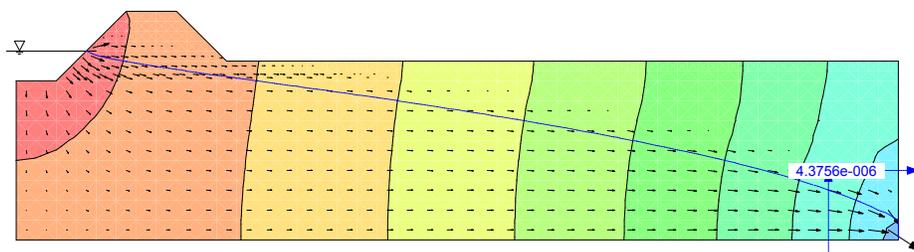
**Figure 2-17 Simulation #2 total head contours ( $K_{sat} = 7.5 \times 10^{-6}$  m/s)**
