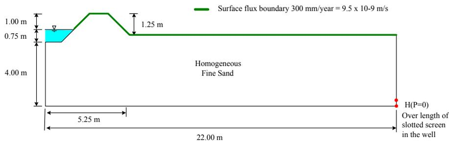
**Figure 2-11 Diagram of system used in sensitivity analysis**
