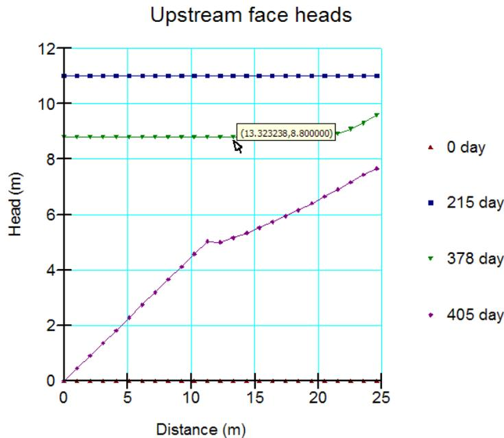
**Figure 7-5 Upstream total head as a function of position for each time**
