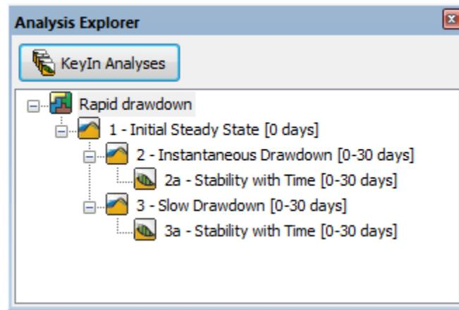
**Figure 4-2 Example of an Analysis Tree in GeoStudio**
