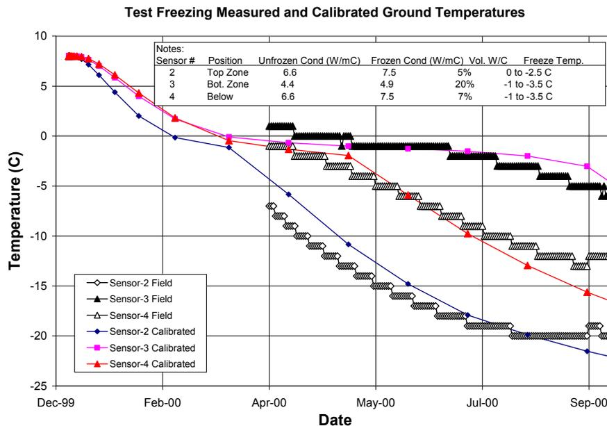
**Figure 2-26 Comparison between actual and calibrated ground temperatures**
