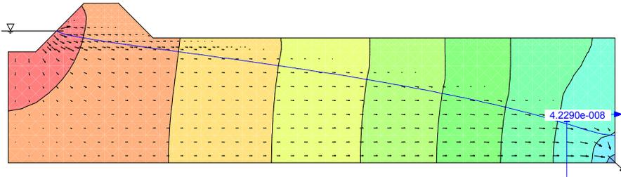
**Figure 2-18 Simulation #3 total head contours ( $K_{sat} = 7.5 \times 10^{-8}$  m/s)**
