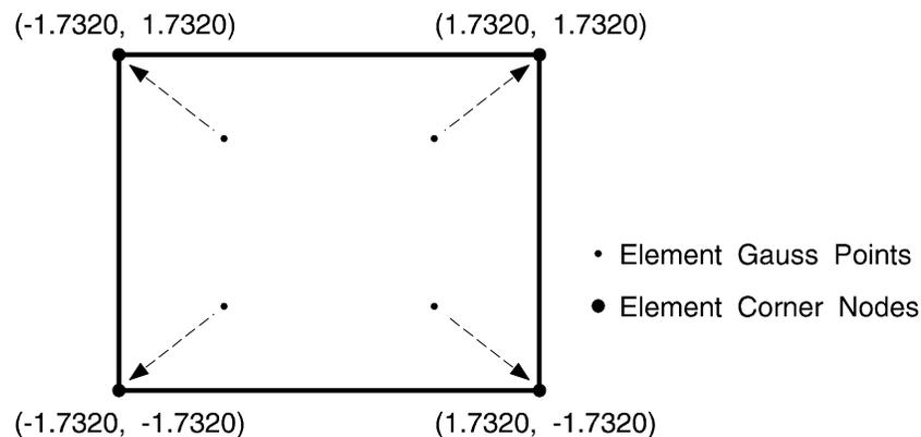
**Figure 7-9 Local coordinates at the corner nodes of an element with four integration points**
