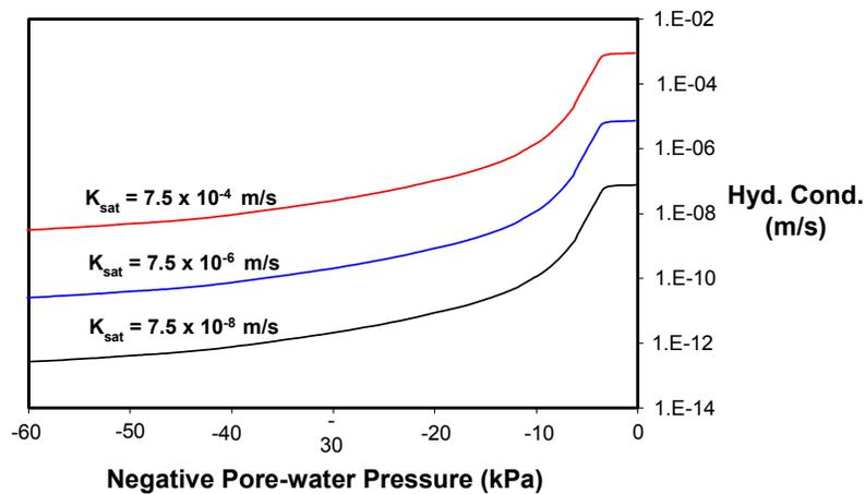
**Figure 2-15 Hydraulic conductivity functions used for  $K_{sat}$  sensitivity analyses**
