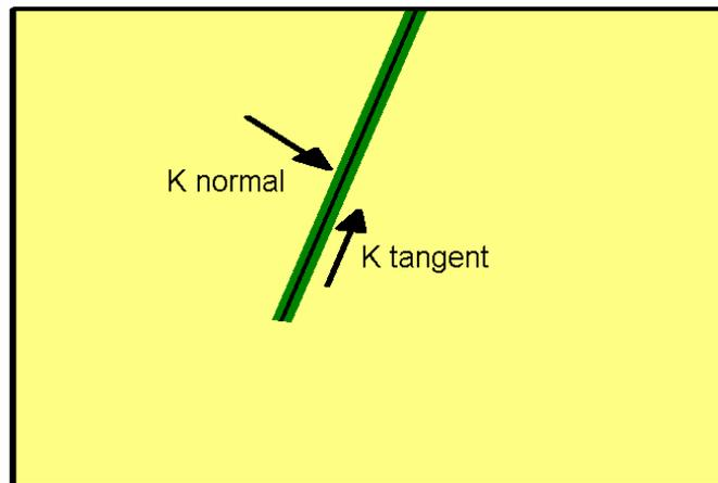
**Figure 2-9 Illustration of interface model assigned to a line**
