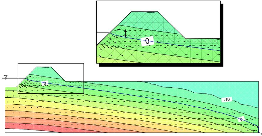
Figure 2-13 Pressure contours and flow vectors for a 3 kPa AEV material
