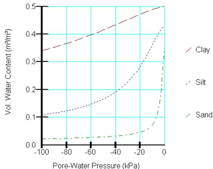
**Figure 2-2 Typical storage functions for 3 soil types**
