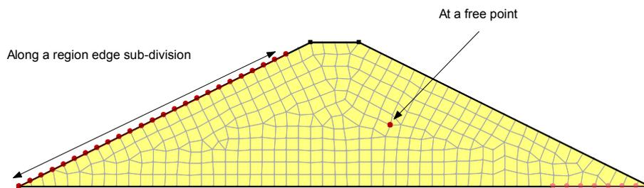
**Figure 3-6 BC's with underlying mesh visible**
