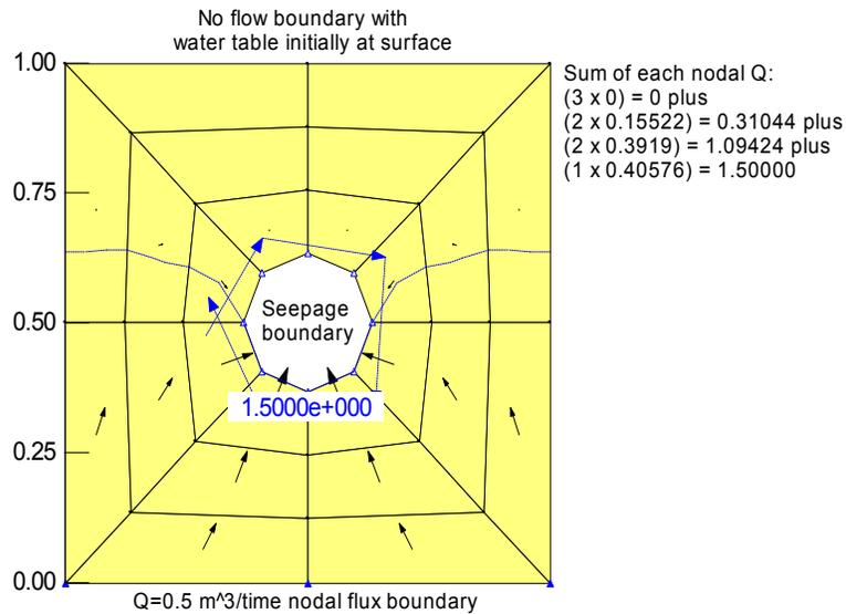
**Figure 7-14 Flux section used around series of drain nodes to check flow**
