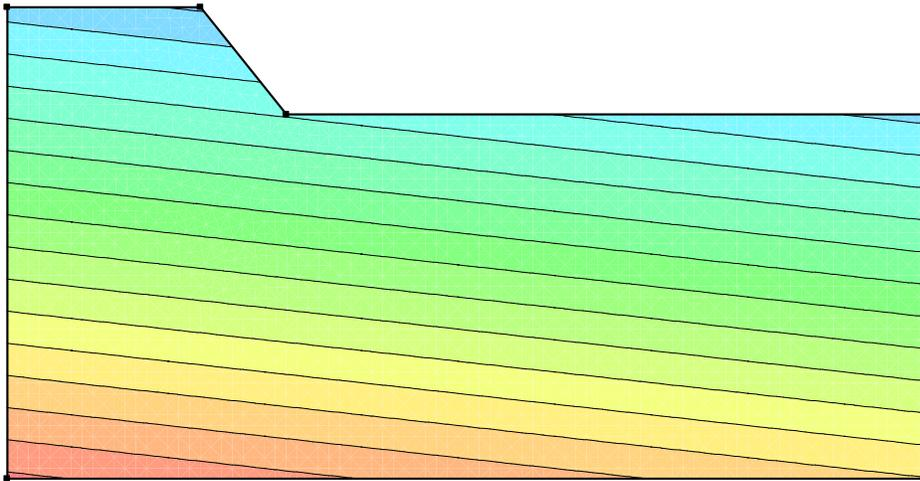
**Figure 4-1 Spatial function assigned for initial pressures**
