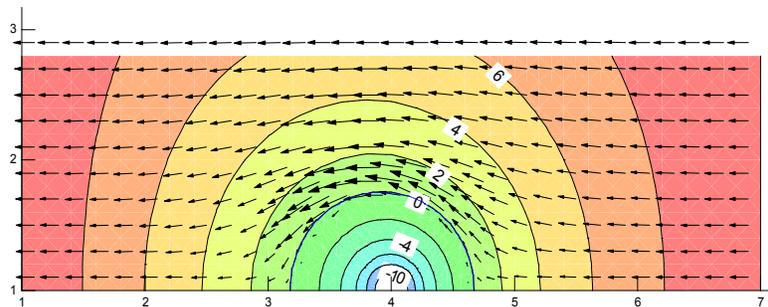
Figure 2-6 Seepage diversion around actively freezing soil region (Temperature contours from TEMP/W displayed)
