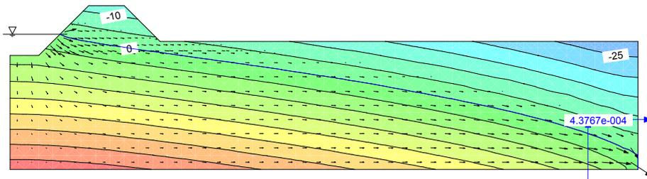
**Figure 2-19 Simulation #4 pressure head contours ( $K_{sat} = 7.5 \times 10^{-4}$  m/s)**
